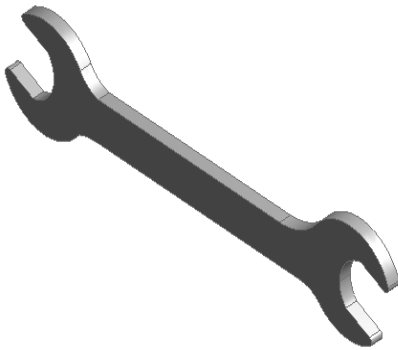
Figure 3-1 Base feature of the spanner
