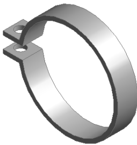
Figure 3-110 Model after creating the circular cutout
