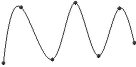
Figure 2-35 Drawing a spline by using the Through Points method
