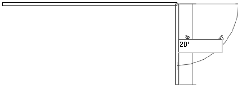
Figure 3-32 Creating the second exterior wall segment
