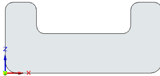
Figure 2-47 Sketch after creating fillets
