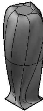
Figure 26-91 Resulting loft feature by using the guide curve
