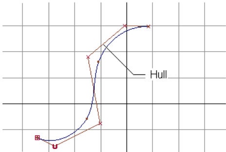
Figure 2-37 Hull of a curve
