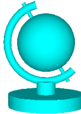
Figure 2-109 Model after hiding the isoparametric curves
