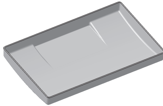
Figure 6-101 Resulting shelled model
