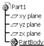
Figure 1-8 The specification tree that appears on starting a new CATPart file
