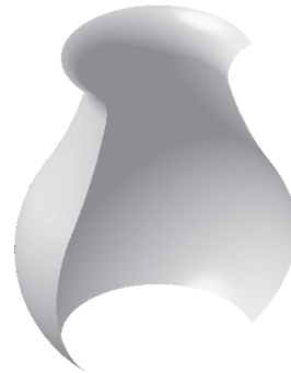
Figure 10-12 Surface revolved through an angle of 180-degree
