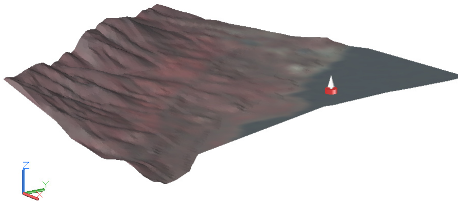
Figure 3-70 The isometric view of the surface with the draped raster image
