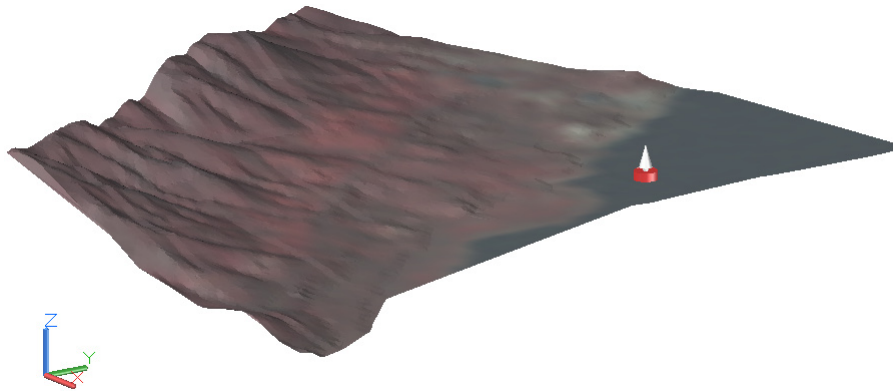
Figure 3-79 The surface with the draped raster image
