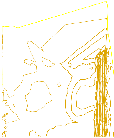
Figure 3-33 Surface contours before using the NNI method
