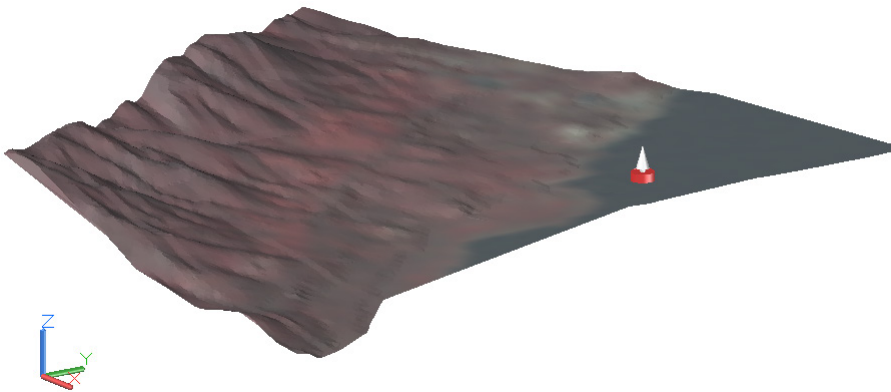
Figure 3-72 The isometric view of the surface with the draped raster image
