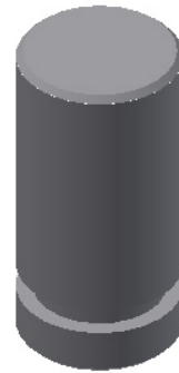
Figure 17-35 The shaft after creating the groove
