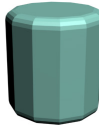
Figure 3-12 A chamfer cylinder with beveled edges
