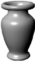
Figure 3-32 The NURBS surface created after using the Revolve tool
