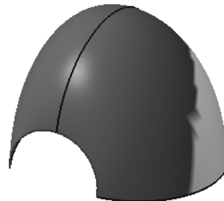
Figure 11-58 The resulting surface created using the Studio Surface tool
