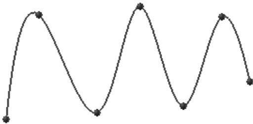
Figure 2-34 Drawing a spline by using the Through Points method
