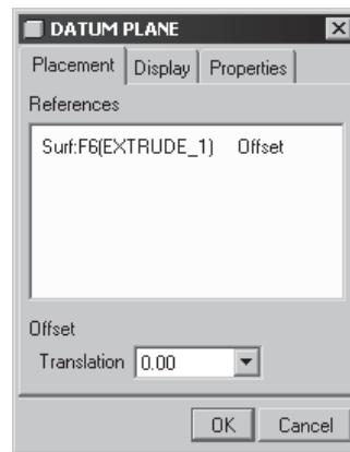
Figure 4-10 The DATUM PLANE dialog box with the Placement tab chosen
