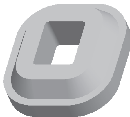
Figure 8-83 Draft applied to all tangent surfaces
