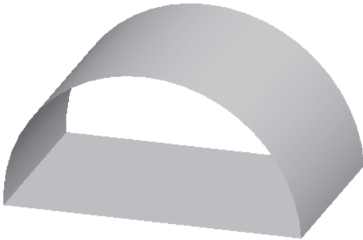
Figure 15-2 Surface with open ends
