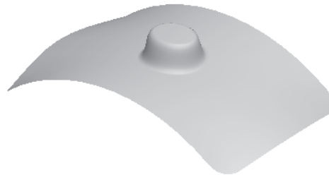
Figure 15-60 Draft offset surface with tangent profile
