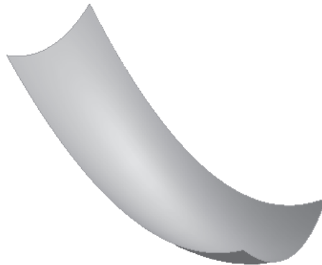
Figure 15-22 Surface created by selecting the curves in two directions
