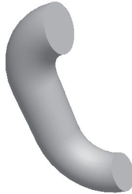
Figure 15-12 Swept blend surface with capped ends
