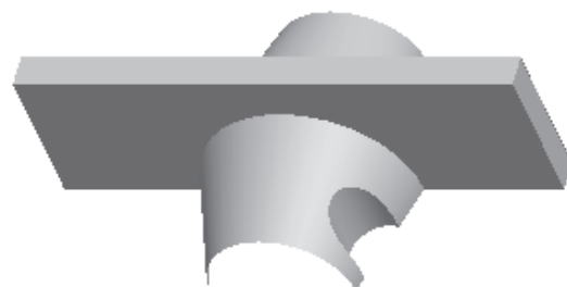
Figure 15-97 Model after merging the surfaces
