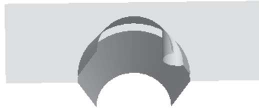
Figure 15-99 Model after merging the mirror copy of the blend surface with the base surface
