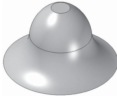
Figure 4-23 Different crown applied to both sides of a protrusion feature
