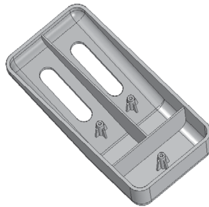
Figure 7-64 Final model after creating the mounting bosses
