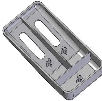
Figure 8-81 Final model after creating the mounting bosses
