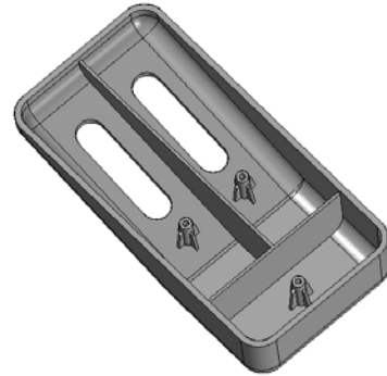
Figure 8-83 Final model after creating the mounting bosses
