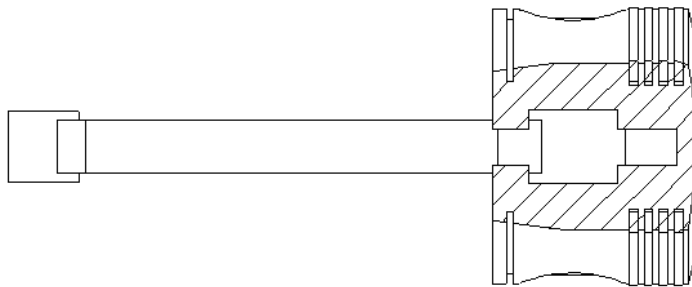
Figure 12-27 Preview of the broken-out section view
