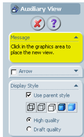
Figure 12-29 Partial view of the Auxiliary View PropertyManager
