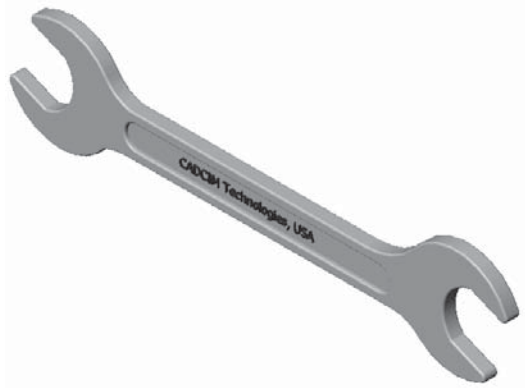
Figure 1-1 Solid model of a spanner
