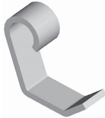
Figure 4-18 Resultant thin feature created with fillets at sharp corners
