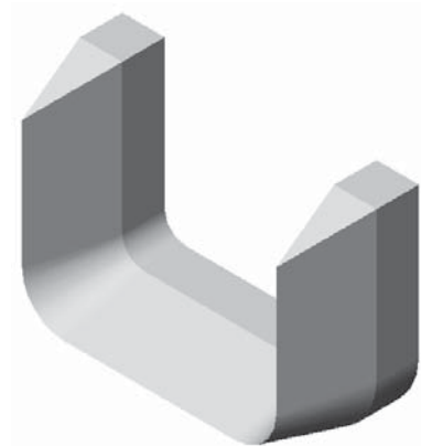
Figure 4-20 Thin feature created in both directions
