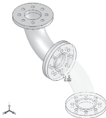
Figure 11-45 Preview of the component being assembled using pattern-based mates
