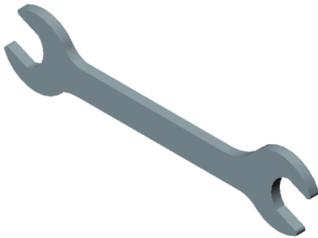
Figure 2-2 Base feature of the spanner
