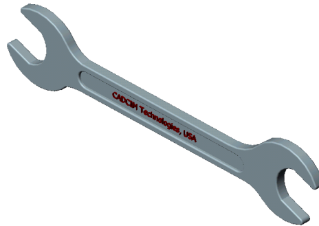
Figure 2-1 Solid model of a spanner
